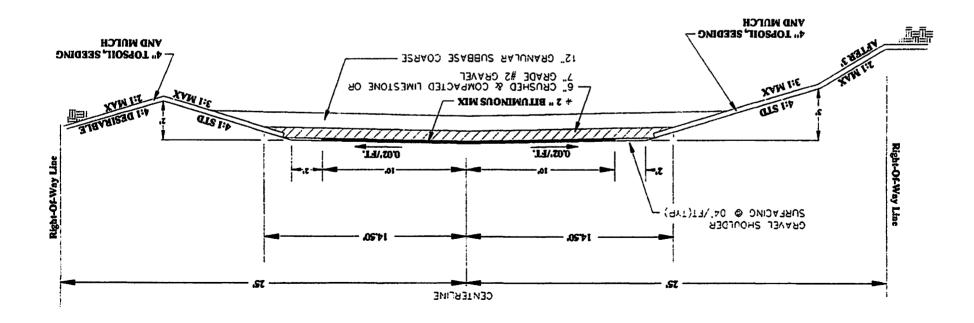
\* EXACT PAVEMENT WIDTHS AND THICKNESSES MAY BE ADJUSTED BY SPECIFIC TOWNSHIP STANDARDS.
